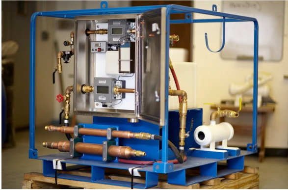
Automatic Foaming Generator (AFG)
