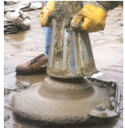
Mix after the addition of AERFLOW with slump of 7-9 in.
