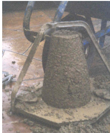
Initial Mix with 1.5 in. slump, before addition of AERFLOW
