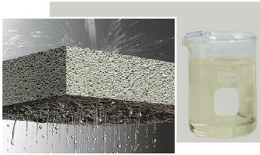
**AQUAERIX™** is an advanced, patented, synthetic foaming agent that utilizes an open-cell technology. AQUAERIX bubbles coalesce creating a capillary-like structure allowing water to pass through. When mixed with a cement slurry, AQUAERIX produces a permeable low-density cellular concrete used in geotechnical applications where increased drainage or reduced buoyancy force is important.
