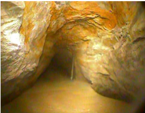
ARX-Transport moving foamed-sand in a dome-out above an abandoned coal mine room.
