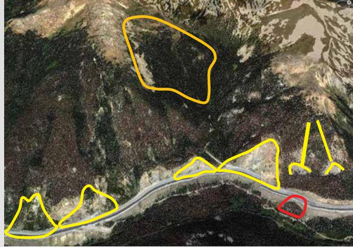
Map of I-70 showing location of landslide features, and slide scars from original construction
