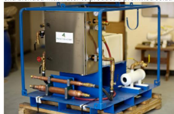
through the foam-making nozzle. No additional water pump is required. The process is completed by air pressure alone. Pressure tanks are supplied in sizes from 30 - 200 gallon capacity to accommodate the project size. Pressure tank generating systems are optimal for operations where batching equipment is utilized. It is very cost effective when relatively small quantities of foam are required.
