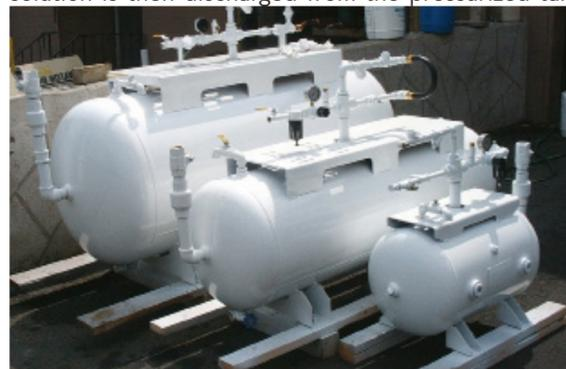
placing equipment, continuous foam delivery is desired, or the volumes of foam required are very large. Aerix Industries™ Auto-Foam Generator (AFG) automatically blends the foam liquid concentrate with water and compressed air in fixed proportions. The AFG continuously siphons the foaming agent directly from the container. The liquid foam concentrate is metered and blended with water to produce a premixed solution
