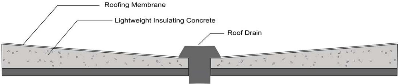
Lightweight Insulating Concrete (without EPS Board)
