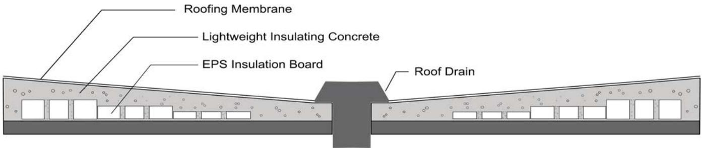
Lightweight Insulating Concrete (with EPS Insulation Board)
